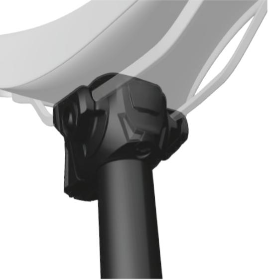
Install the saddle and left and right saddle retainer caps to hold the saddle rails.
